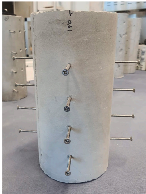
Fig. 3. Image of sample with embedded probes. Embedded probes installed in accordance with AASHTO Designation T359-19 surface measurement locations at 0°, 90°, 180° and 270°.
