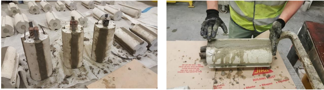
Figure 1 – Concrete sample anode installation
