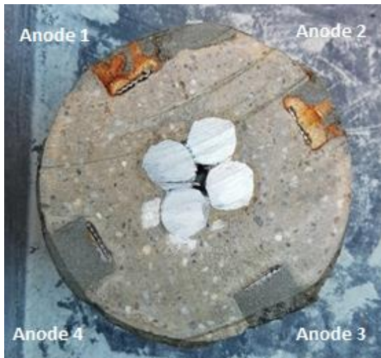
Figure 7 – Experiment 2, cross section of sample at the point of water ingress below water level
