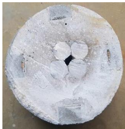
Figure 2. No water ingress to anode locations
